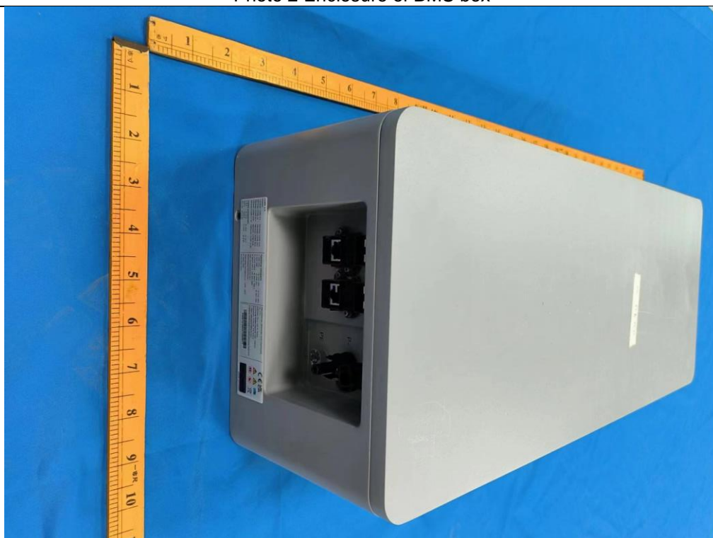
Photo 3 Enclosure of BMS box
