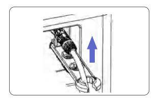
5. Remove the screws between BMS and the battery stack. And then lift the BMS from the tower.
