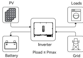
When the load consumption exceeds the  $P_{max}$ , the inverter will take power from the battery and PV to supply power to the load to compensate for the power that exceeds the  $P_{max}$ .
