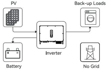
When the power from PV isn't enough, the battery will discharge to supply back-up loads together with PV.
