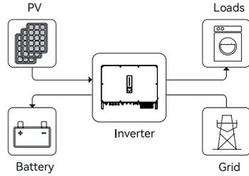
When the grid fails, power from PV and battery will supply loads connected on the back-up side (UPS).
