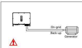
The on-grid and back-up side cannot be connected to and generator directly. For advanced applications, please contact our after-sales department.
