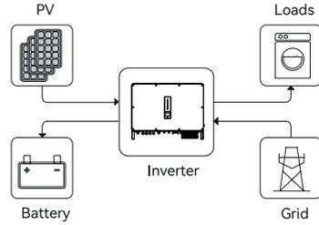
Inverter will use power from PV and battery to supply loads in the predetermined period and the insufficient part will be supplied by the grid.
