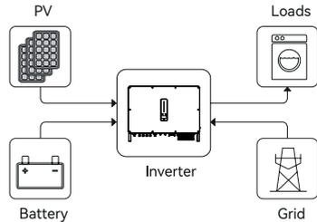
**Peak load Shifting (Load Shifting)**
