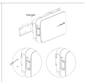
⑥ Lift the inverter. Align the inverter's bracket bolts with the grooves on the inverter bracket. Move downward first, then to the left, to slide the bracket bolts into the grooves. Tighten the M5 screw on the right side to secure the inverter.
