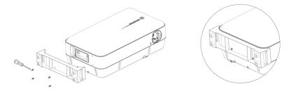
② The floor-standing bracket is composed of three components. Assemble these components together using screws.
