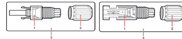
1. Insulated Enclosure 2. Lock Screw 3. Positive/ Negative Connector
