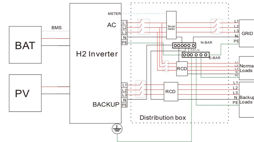
The system connection for grid system without special requirements is as below.
