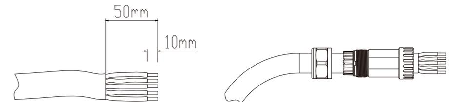
(3) When connecting cables, the AC cables should be tightened and fixed with a hex wrench according to the wiring labels L1, L2, L3, N and PE .
