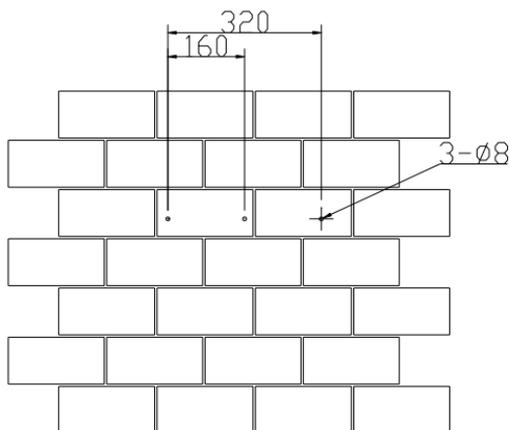
Figure 4.8 Drill holes' dimensions of R5-17K/20K-T2
