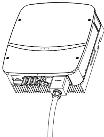
Figure 5.11 Tighten up AC interface protective cover and the locker
