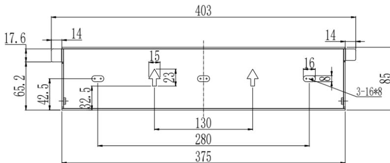
Figure 4.4 Dimensions of rear panel of R5-13K/15K-T2
