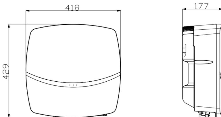
Figure 3.2 Dimensions of R5-3K/4K/5K/6K/8K/9K/10K/12K-T2
