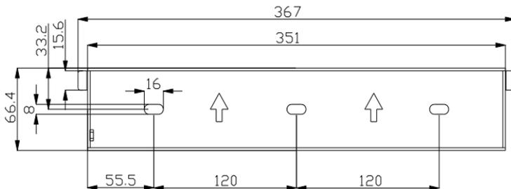
Figure 4.3 Dimensions of rear panel of R5-3K/4K/5K/6K/8K/9K/10K/12K-T2
