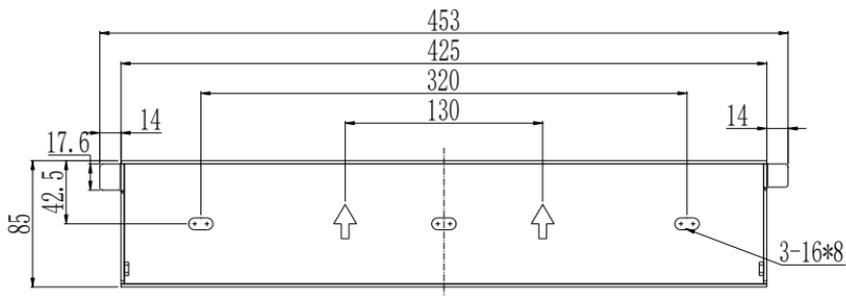
Figure 4.5 Dimensions of rear panel of R5-17K/20K-T2
