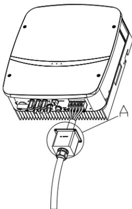
Figure 5.10 Connecting the cable
