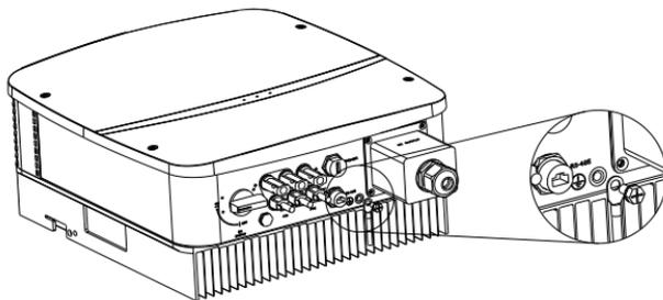
Figure 5.9 Inverter ground protection
