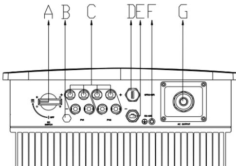
Figure 5.3 Electrical interface of R5-17K/20K-T2
