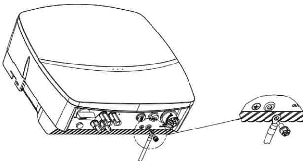
Figure 5.4 Inverter ground protection
