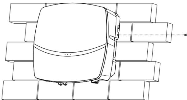
Figure 4.11 Fasten the inverter and hanging panel with screws
