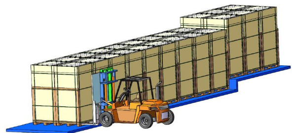
Long-side vertical package unloading with forklift
