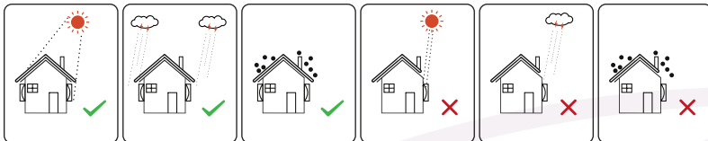
Figure 4-1 Recommended installation location
